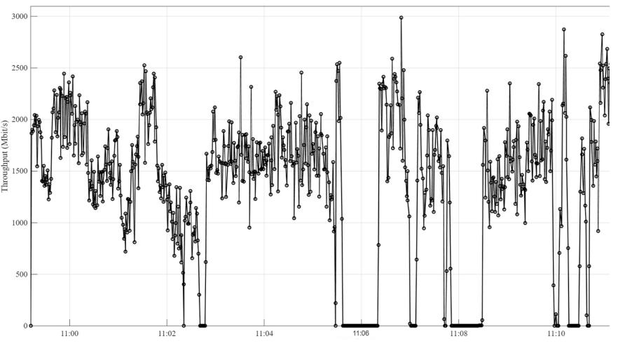
The 26 GHz (mmWave) band achieved peak throughputs over 2.5 Gbps, delivering very high capacity but showing greater variability depending on LoS conditions and antenna alignment.
