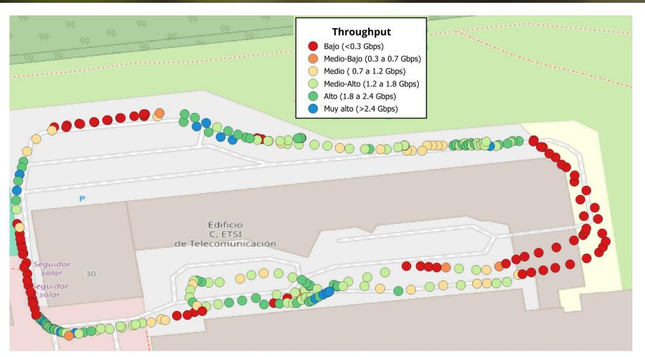
The map shows the 26 GHz throughput along the drive route, highlighting strong correlation between high data rates and line-of-sight coverage from the mmWave sectors.
